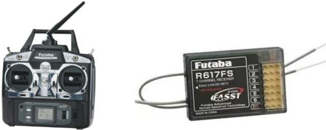
Figure 2.4 Futaba RC transmitter and receiver.
