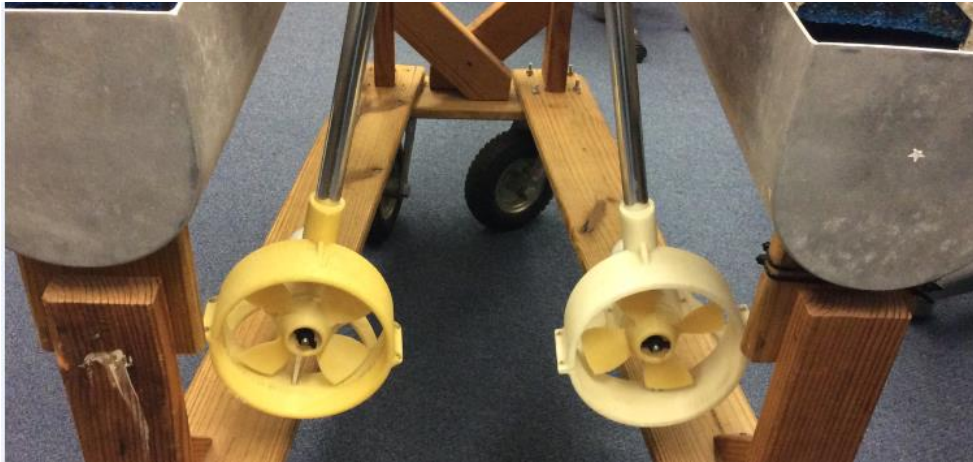
Figure 2.11 The ASV propellers and shrouds system.
